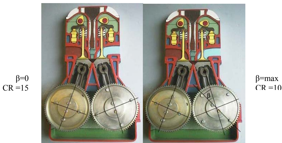
Figure 12: The “CVCR” engine with self-adjusting compression ratio
