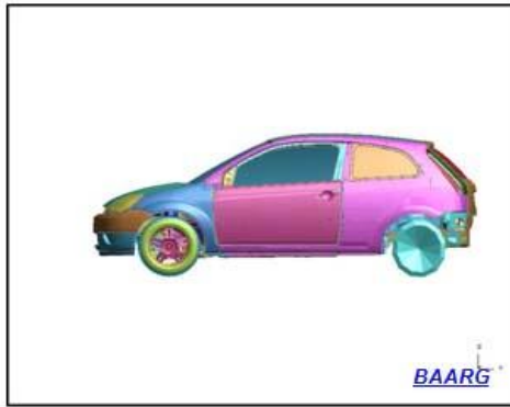
Figure 2: Ford Fiesta developed model for against virtual testing
