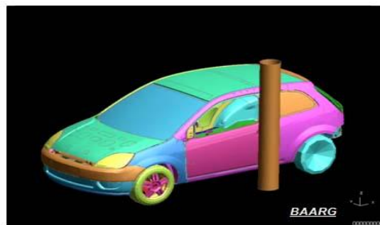
Figure 5: The Ford Fiesta under pole impact
