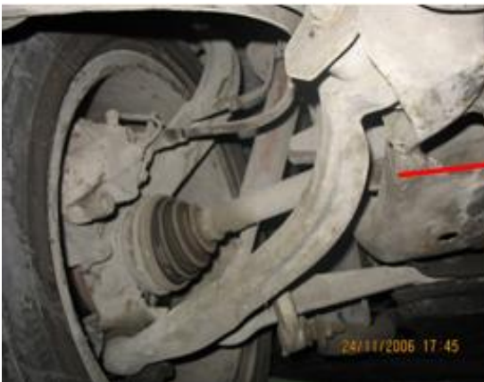
Welding traces at front axle
