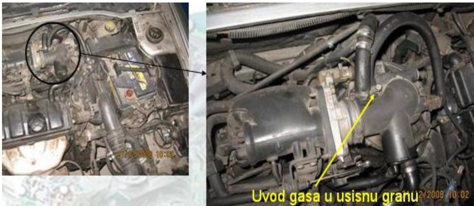
Vehicle manufacturer built-in LPG device replaced with un-original one
