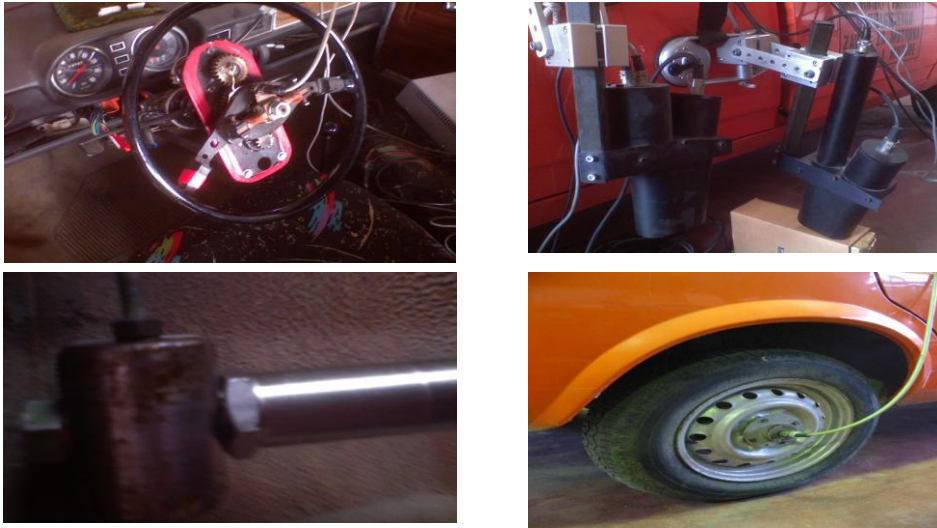
Figure 4: Vehicle experimental systems for tire/road friction estimation
