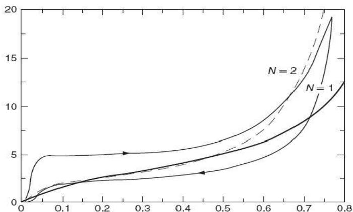
**Figure 8:** Nonlinear characteristic for flexible polyurethane foam [12]
