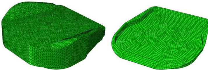
**Figure 7:** The meshed model of seat cushion
