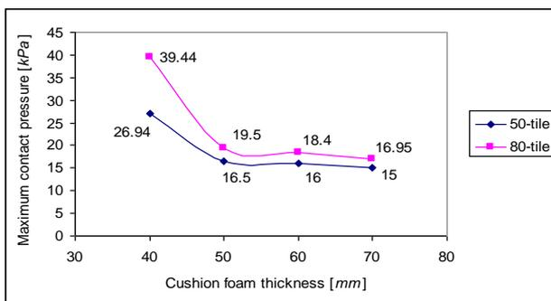
Figure 12: Relationship of maximum contact pressure and seat cushion thickness
