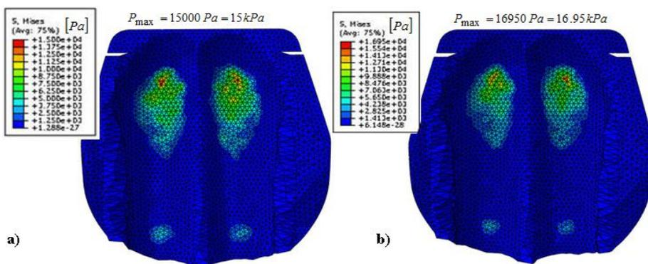
**Figure 11:** Pressure distribution on the contact surface of virtual seat cushion and virtual model of human from; a) 50th and b) 80th percentile
