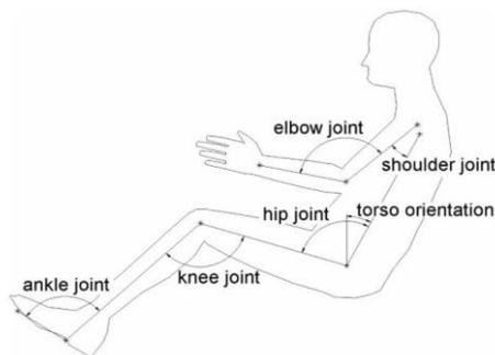
**Figure 1:** Parameters of driver’s work position [17]
