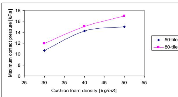
Figure 13: Relationship of maximum contact pressure and density of the polyurethane foam
