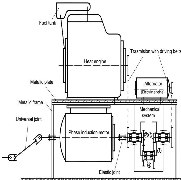
**Figure 6:** The constructive scheme of the prototype
