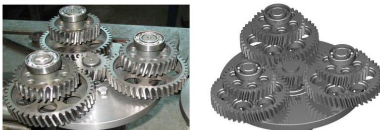
**Figure 7:** The image obtained with a camera (left) and the photographic representation in AutoCAD of the gear mechanism (right).
