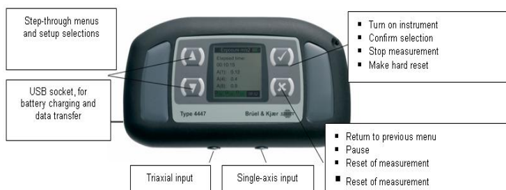
Figure 9: The four buttons on the front panel control the user interface of Type 4447
