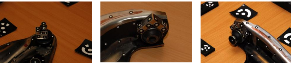
Figure 3: Application of cylinder adapters in digitizing project
