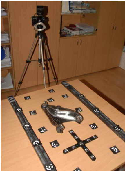
Figure 4: Individual measurement by optical measuring system TRITOP
