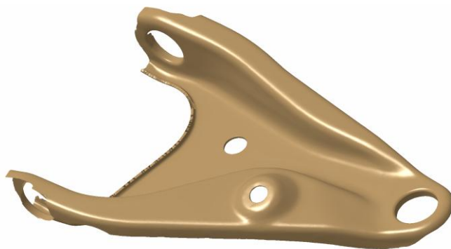
Figure 10: Poligonized mesh constructed over a generated point cloud
