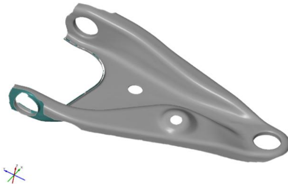
Figure 8: Poligonized mesh constructed over a generated point cloud
