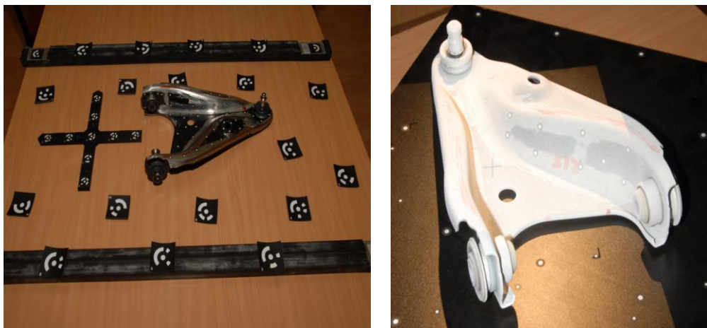
Figure 1: Measuring volume prepared for optical measurements by optical measuring systems TRITOP (left) and ATOS (right)
