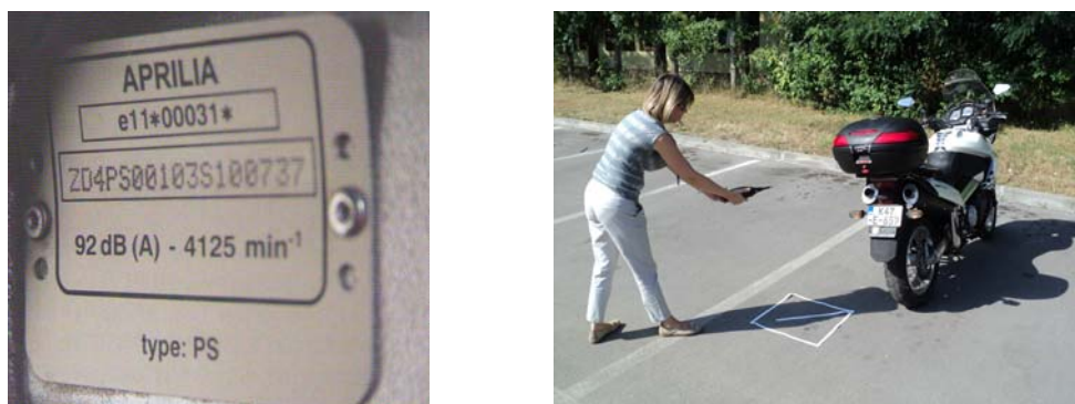
Figure 3: a) Identification label, b) motorcycle and microphone position at the test site
