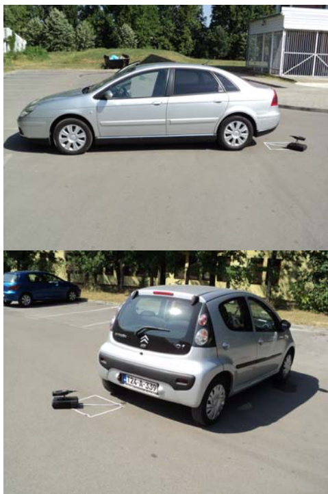
Figure 4: Position of cars at the test site and a microphone position
