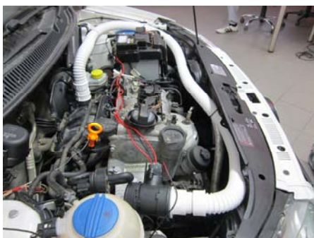
Figure 15a: Air mass meter and intake hose installation setup
