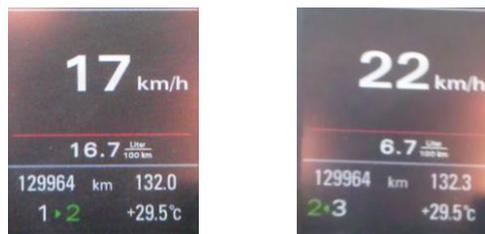
**Figure 5** Gear change indicator – Audi A4 B8
