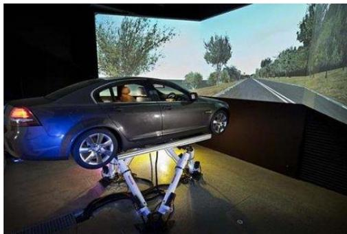
**Figure 8** *Driving simulators*
