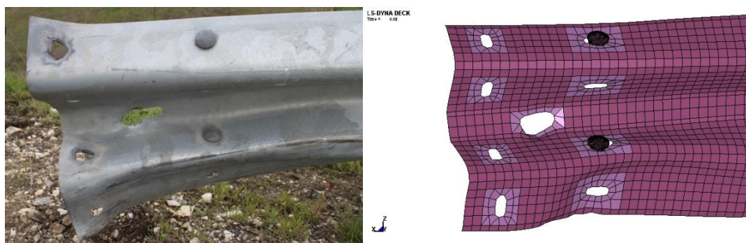
Figure 4. Real and FE segment deformation mode
