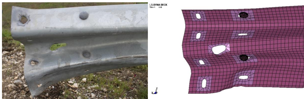
Figure 4. Real and FE segment deformation mode
