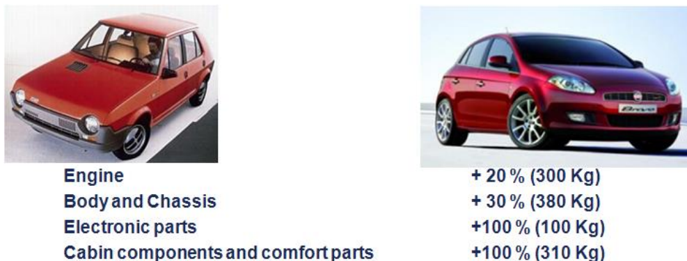
Figure 3 – Evolution of the vehicle weight for a FIAT medium size car
