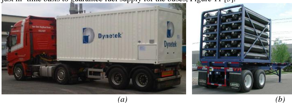
Figure 11: The 300 bar Modules (a) ISO 20 ft Container (b) 10 ft Cube for Bulk Transport of CGH 2
