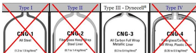
Figure 8: Comparative analysis of the (mass/volume) ratio of various cylinder types (example CNG cylinders)
