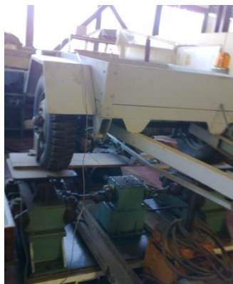
Figure 3 Two single axle trailers for road profile measurement on the experimental stand and towed by experimental “vehicle 1”
