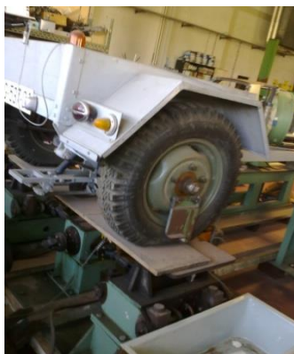
Figure 3 Two single axle trailers for road profile measurement on the experimental stand and towed by experimental “vehicle 1”
