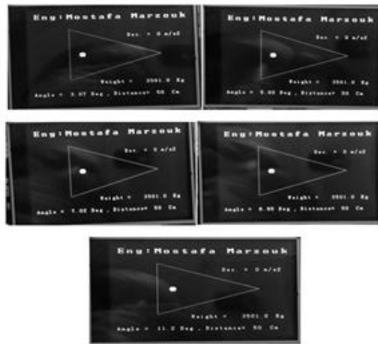
Figure 14 Forklift C.G. position at different road inclination angles
