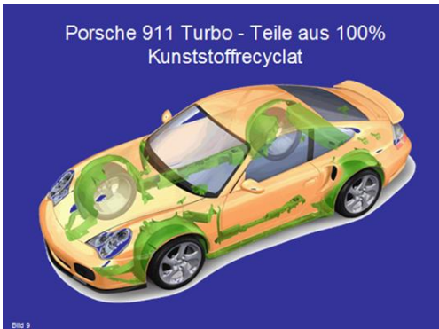
Figure 7. Plastic parts from recyclates in Porsche 911 Turbo
