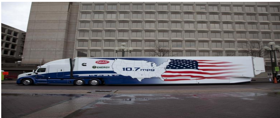
Figure 8. The US class 8 tractor trucks for heavy working conditions with Cummins engines and Peterbilt equipment with intention to achieve 10.7 miles with one gallon under real driving conditions. The truck was inspected by the Department of energy (Source: Photo Sarah Garrity)
