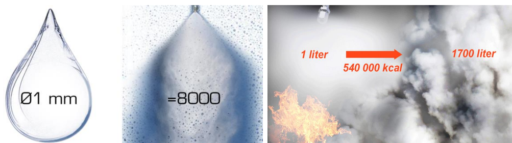
Figure 9. Normal sized water drop vs. water mist and extinguishing fluid water mist effects
