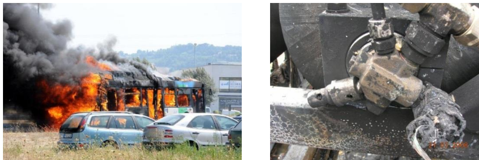
Figure 4. CNG bus under fire (left) and PRD which were successfully activated in a fire (right)
