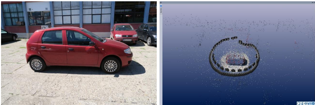
Figure 2 and 3. Undamaged vehicle and generated cloud points with camera positions at the moment of recording
