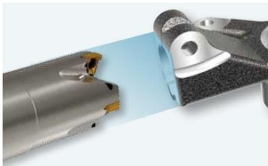
**Figure 16.** Face roughing and finishing [8]
