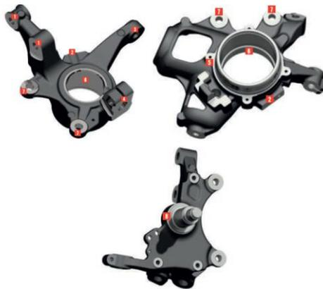
**Figure 9.** Surfaces operation machining [20]
