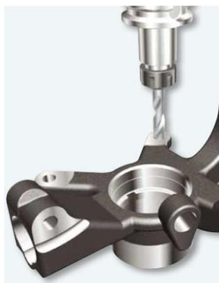
**Figure 11.** Drilling [8]
