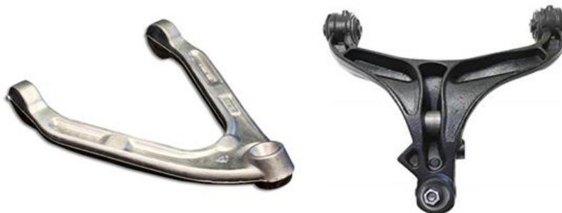
**Figure 6.** Forged control arm [5, 13]
