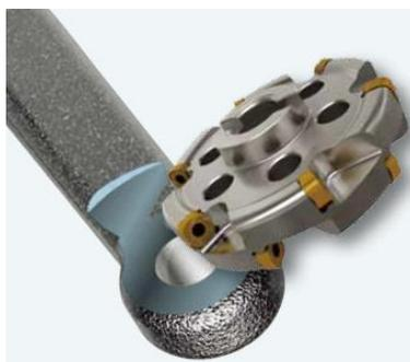
**Figure 12.** Full side face milling [8]
