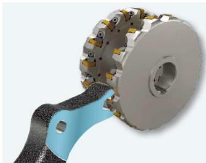
**Figure 10.** Double side milling [8]
