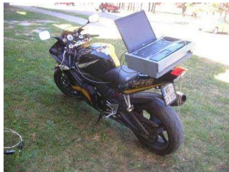
Figure 7: The measuring system HBM Spider 8
