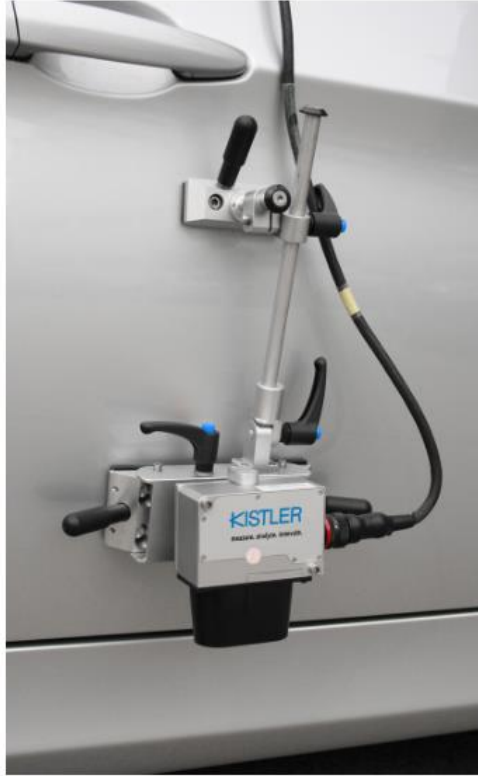
Figure 6. Preferred way of mounting during testing
