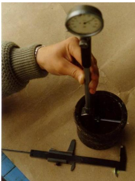
Figure 4 Methodology for measuring the shoe sleeve
