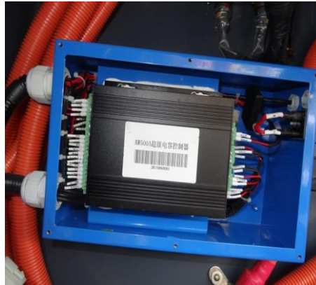
Figure 3 BMS control unit
