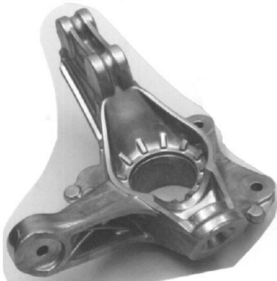
Figure 2 Appearance of steering knuckle [11]
