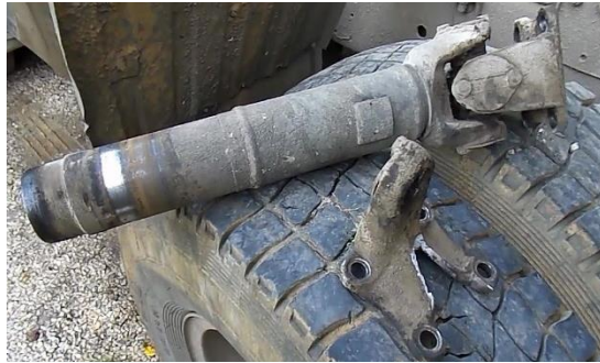
Figure 3 Failure of the driveshaft
