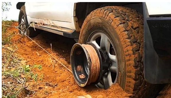
Figure 4 Method of using the rope-block device
