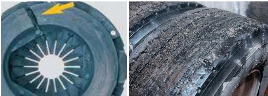
Figure 2 Fracture and overheating of the pressure disc with constant slippage of the clutch
