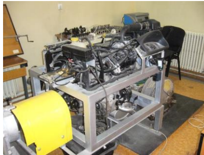
Figure 13 The test bed used to obtain the indicator diagram
