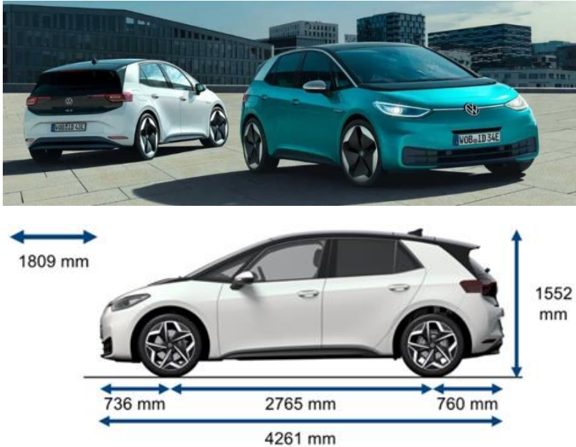
Figure 2. Appearance and dimensions of the adopted EV [21,22]
