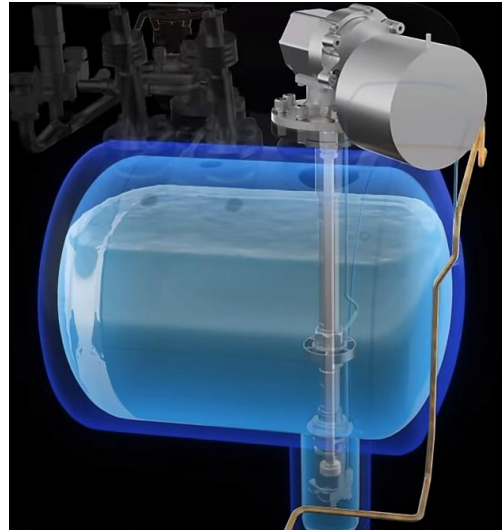
Figure 8 Toyota GR Corolla with lately introduced liquid hydrogen storage with cryogenic pump [83]
