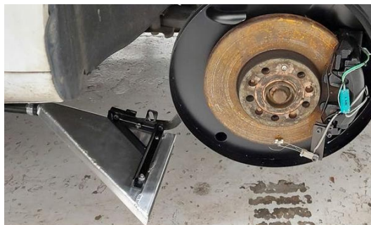
Figure 14 Variants of devices on vehicles for drawing in and measuring particles produced by tire wear in case of road tests, a) first variant, b) second variant, c) third variant [36, 37, 38]
